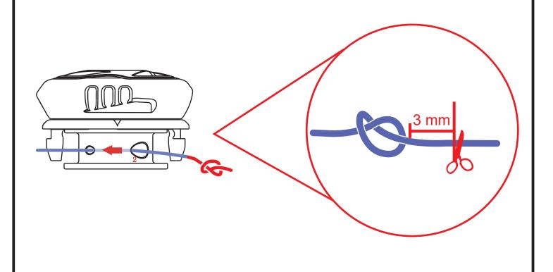
(4) Thread wire's terminal back to hole 2 to the bottom
