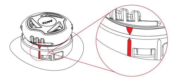
4. Hold firmly the knob and pull it up to disassemble it from the base.
