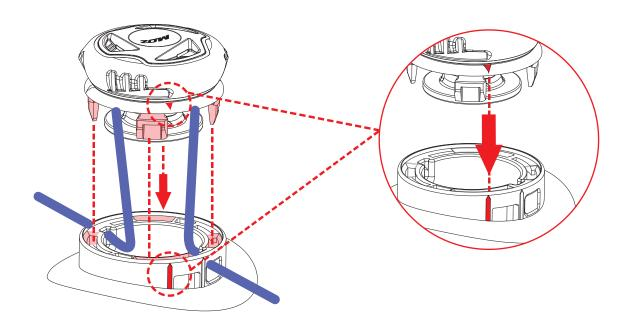
(2) Turn the knob on the counterclockwise, and ensure that the arrow on the top knob and the one on the base are aligned. After you hear the "Click" sound, this means that the procedure is done.
